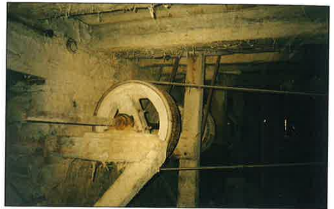
Fig. 9. Water powered wood working workshop – driving belt system.
