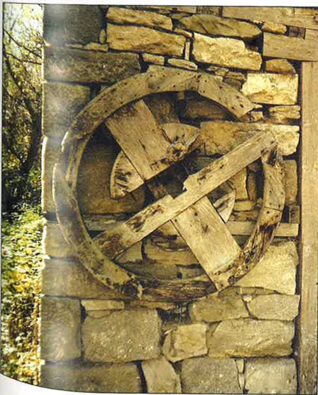
Fig. 10. Water powered wood working workshop – wheel of the carriage driving mechanism.
